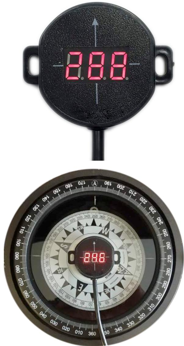
C20-00132 is used to convert the magnetic field to NMEA0183 output signal.
